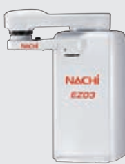
Floor mount type Z-axis 250mm EZ03F4-5525
